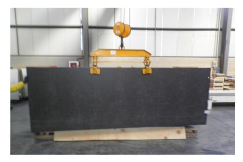
The additional width of the clamp will prevent the slab from bending and twisting when transporting and thus avoiding unwanted ruptures. In the case that this type of clamp is not readily available, the following recommendations will adapt existing clamps to handle Neolith slabs without any problems.
